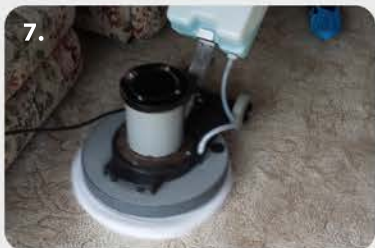
7. Rotary absorption - Absorb and warm carpet fibres to remove as much excess moisture as possible to speed drying.
