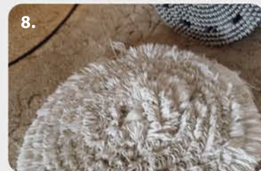
8. Check bonnet - Inspect bonnet to ensure complete removal of soil.
