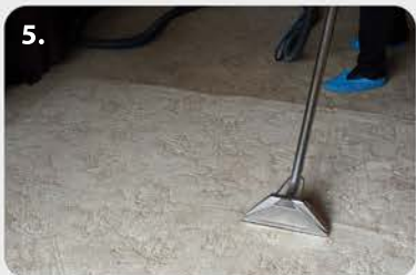
5. Neutraliser rinse - Rinse and extract all broken soils in fibres with appropriate rinsing solution to ensure correct PH level of fibres.
