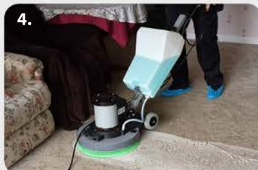
4. Combination - Rotary agitation.
