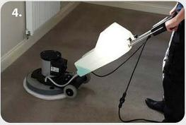
Bonnet Absorpotion - bonnet fibres with rotary machine with fibre shampoo.
